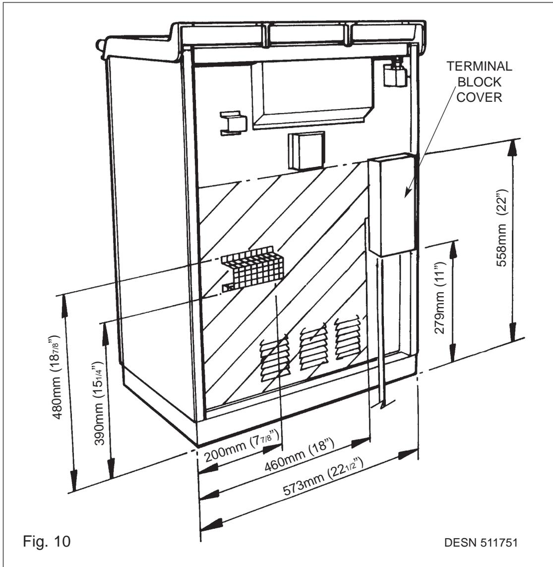
The gas flexiline connector must be fitted in the shaded area indicated in Fig. 10. Take into account that it must be possible to pull the cooker forward sufficiently and that no strain occurs on pipework. Ensure flexiline is not trapped between electrics cover and rear wall. Ensure flexiline is routed within shaded area, and away from the shielded vent.
