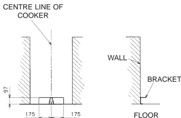
To reduce the risk of tipping, the range must be secured by a properly installed anti-tip bracket supplied with the range. The bracket must be fitted within the shaded area shown in the diagram using 2 x screws (No.10 x 1 1/4") fixed in the wall or floor, longer screws may be required depending on the wall or floor covering.
