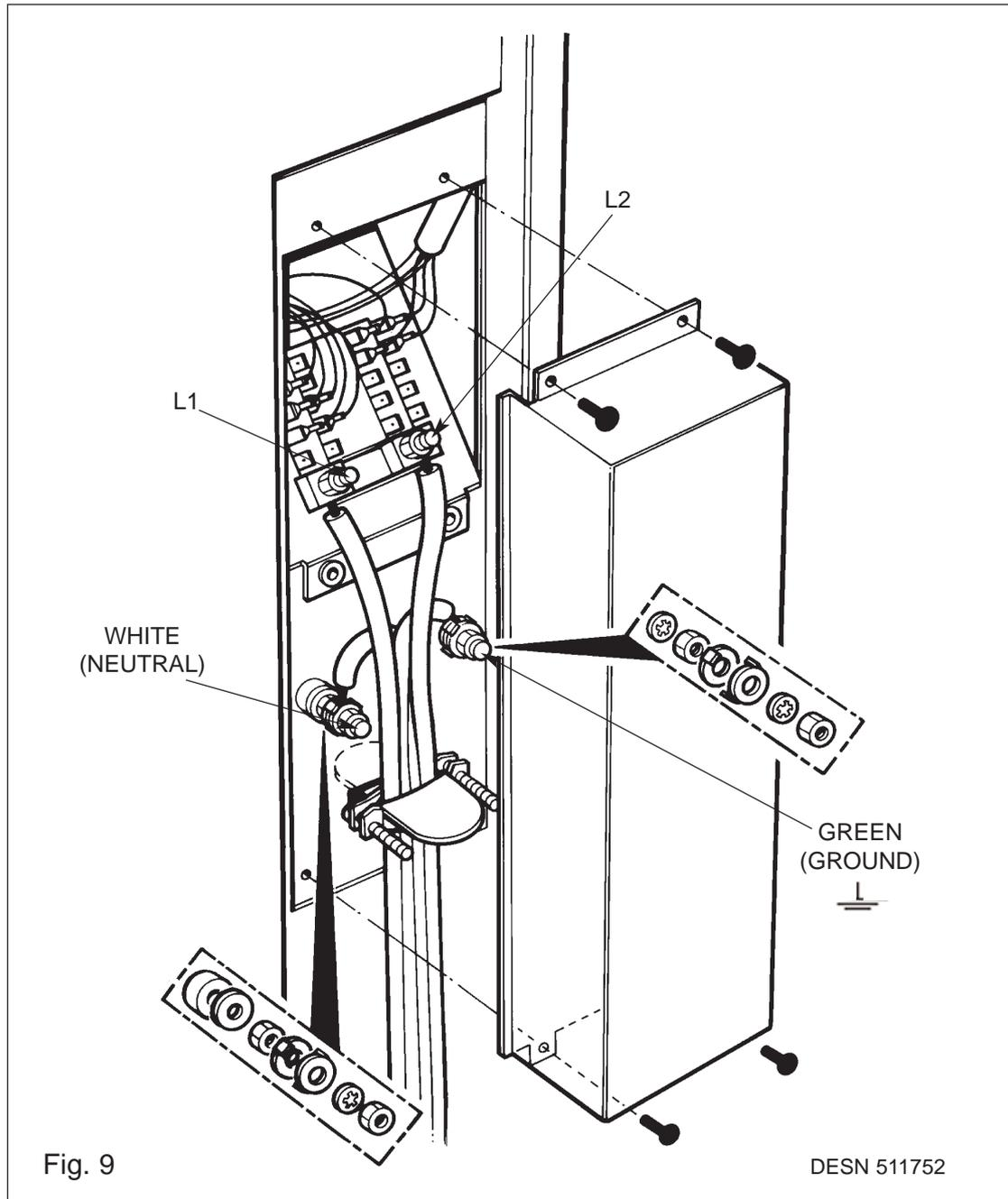
1. Assemble a U.L.-listed strain relief in the opening.
