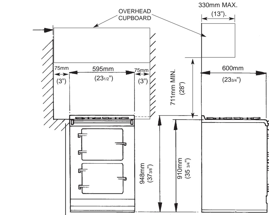
**APPLIANCE CAN BE CLOSE FITTED TO KITCHEN UNITS UP TO WORK TOP HEIGHT.**
